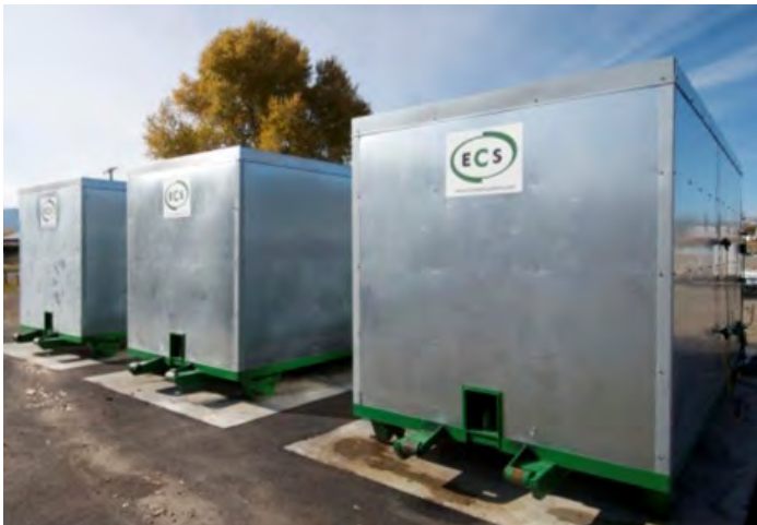
Engineered Compost Systems (ECS) - Large Container Type In-Vessel Composting (Photo by ECS)
